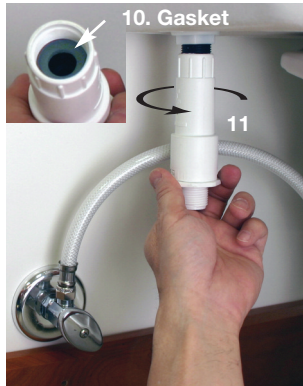
10. Make sure gasket is seated at base of threads in the EXTERNAL REGULATOR. 11. Thread EXTERNAL REGULATOR onto lower supply shank and hand tighten.
